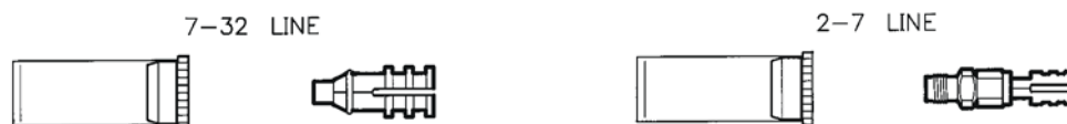
Figure 1-6 Line Standards — 7 to 32 GHz and 2 to 7 GHz Air Lines Installed in Tools with Storage Bottles
